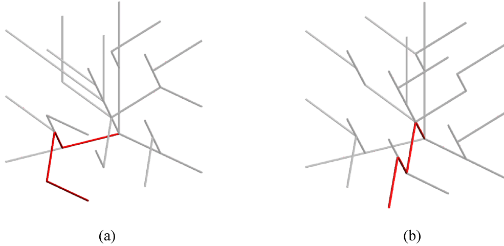
Figure 3.1.6: Comparison of the configuration obtained by means of the adapted algorithm (a) and the optimal configuration (b) in case of an ensemble of 35 tetrakaidecahedra. For the sake of clarity, only cell center connections are displayed here.
