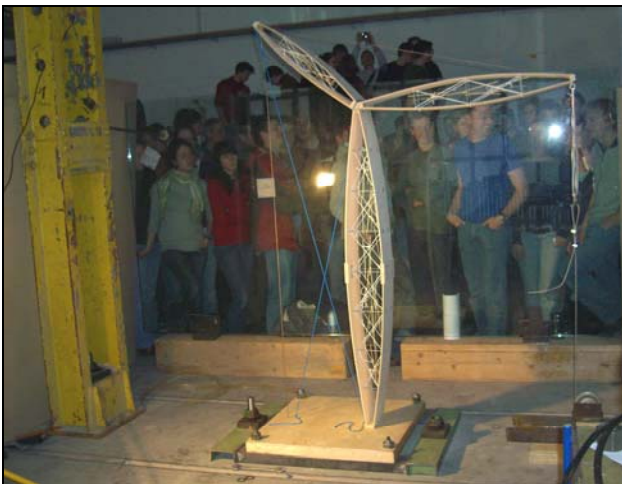
Figure 7: Student Project "Crane in the Bag" – Testing of Tower Crane
