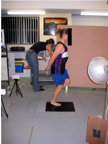
Figure 10: Hopping test to assess musculotendinous stiffness on a force plate. (own material)
