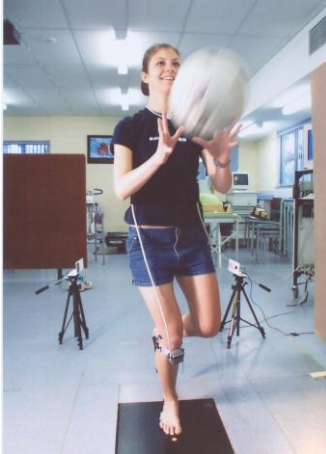
Figure 6: A subject landing on the designated area (force plate) while catching a netball. In the background the timing lights can be seen. (own material)
