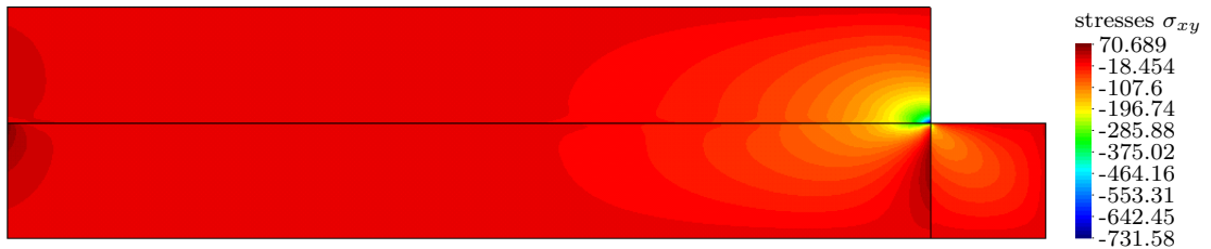
Figure 5.49: Tangential shear stresses \sigma_{xy} for pure stick case.
