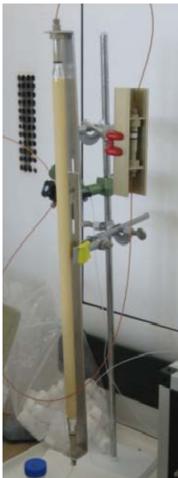
Fig. 26: Manually assembled separation column
