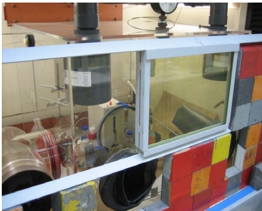
Fig. 42: Glove box in which highly enriched ^{176}\text{Yb} targets were processed; for the picture, lead bricks were removed on the left side
