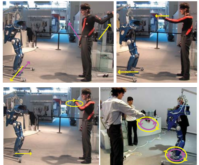
Fig. 13. Human gesture commands and corresponding robot's gait primitives: (top left) side walk right/left, (top right) go back, (bottom left) come, (bottom right) turn clockwise/counterclockwise.
