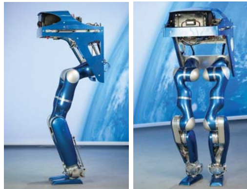
Fig. 1. DLR-Biped: A biped walking machine with torque controlled joints.
