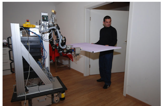
Fig. 2 Joint manipulation task of a human and a robot using haptic interaction
