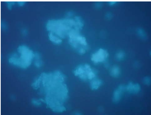
Fig. 15. PVPP particles exhibiting auto fluorescence.
