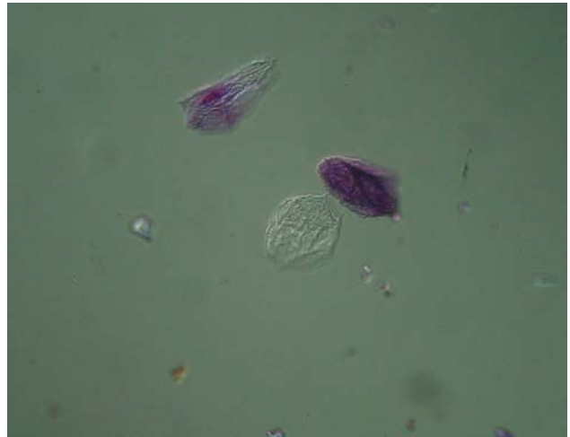
Fig. 6. Haze made of polysaccharides stained with Thionine.
