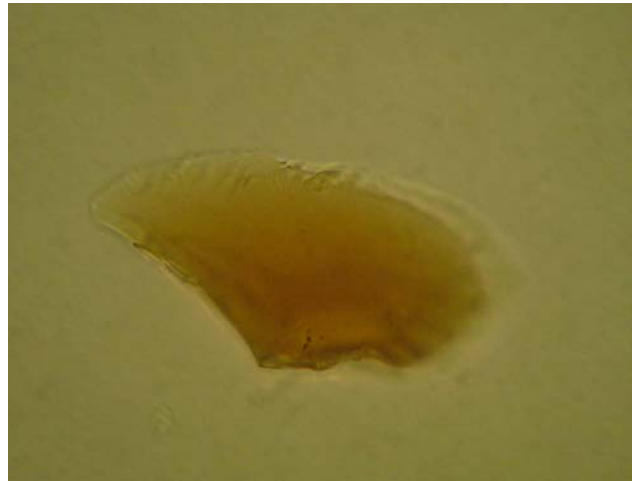
Fig. 22. Glass particle in a transmitted light beam.
