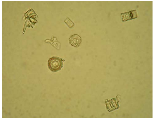
Fig. 17. Kieselguhr particles in a transmitted light beam.
