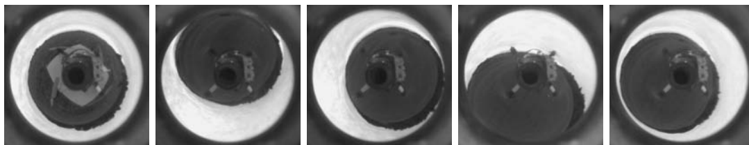
Figure 1.2: This sequence shows images acquired by a catadioptric camera mounted on a quadcopter. It would be straightforward to extract the horizon (note the slight irregularities and texture differences) which could then be used to estimate the full rotation and not only the yaw angle (visual compass).
