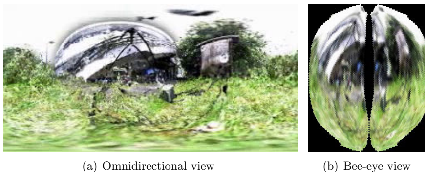
Figure 1.1: The left image shows an unwarped omnidirectional view rendered from the data acquired by a Z&F laser-scanner. The right image shows the same view as seen through the eye of a bee. (Both images are by courtesy of Wolfgang Stürzl [30])
