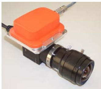
Figure 8.38: A PointGrey Flea2G camera with wide angle lens and a Xsens-MTi IMU (orange box) as it is used in our experiments.
