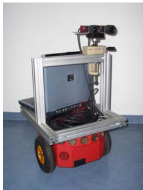
Figure 8.27: Experimental setup: a Pioneer3-DX equipped with two Marlin cameras.
