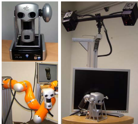
Figure 9.3: The upper left-hand side picture shows the DLR 3D-Modeler with the IMU module and the PC running the software. The other two images demonstrate each a global registration variant for the scan device: a robot arm ( lower left ), and an external tracking system ( right ).
