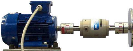
Figure 6.7: Setup for closed-cycle efficiency evaluation: Induction machine with torque transducer and flywheel.
