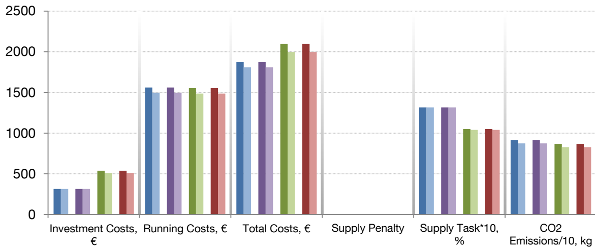
Figure 5.15 Costs, emissions and supply task fulfilment. Exhaustive search optimization results for CBo1 and CBo2 (Table 5.1). Supply task is satisfied, although also exceeded (overproduction) in case of saving on investment costs. Moscow, “S” building.
