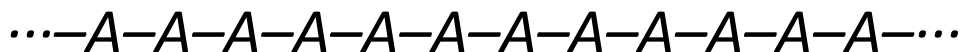
Figure 1.1. Representation of an homopolymer which contain the same type of monomers (A) bonded together.
