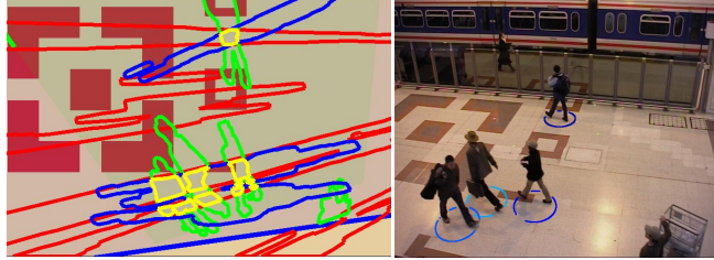
Fig. 3. Detection example applying homographic transformation in the ground plane. Detected object regions are subsequently projected into the third view of the PETS2006 data set. The regions in yellow represent intersecting areas. As can be seen, some objects are split into multiple regions. These are aligned in a subsequent tracking step.
