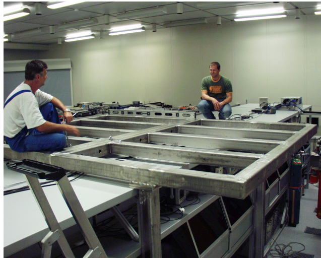
Figure A.6: The bridge seems stable enough for a first static load test.
