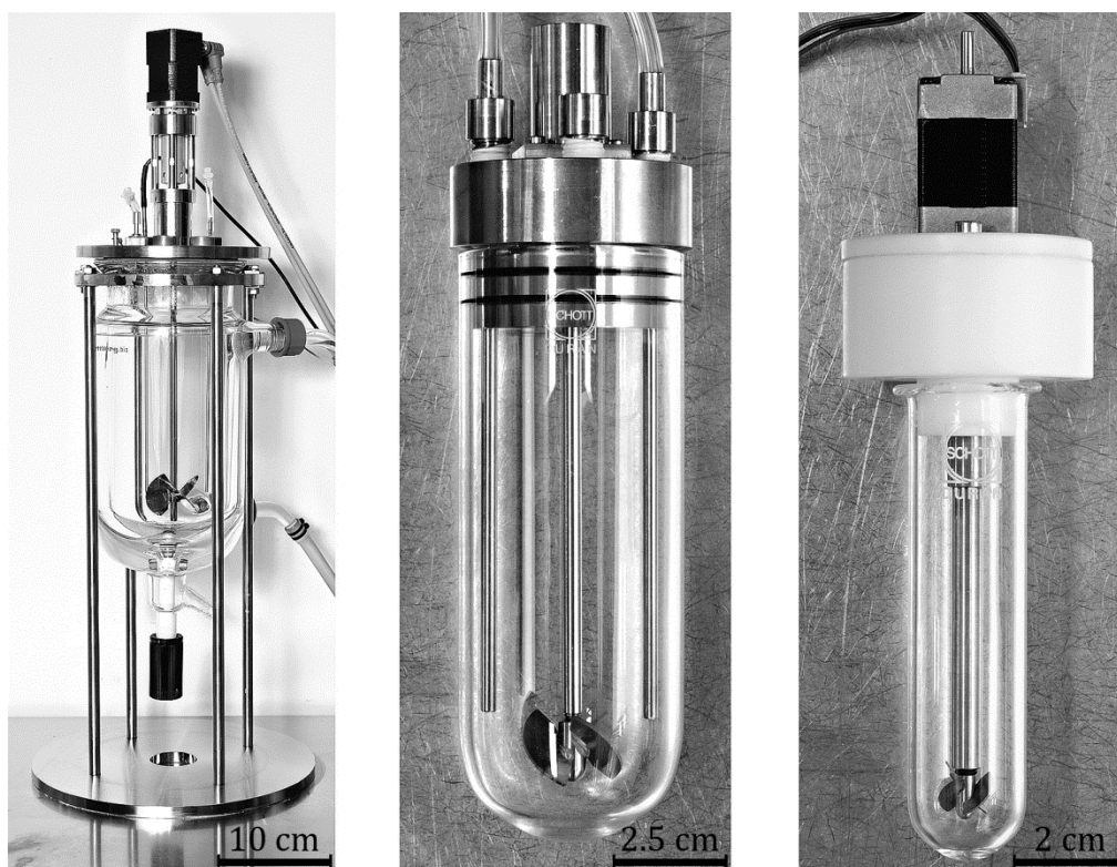
Figure 4.2: Geometrically similar stirred tanks used for the agitated batch crystallization on a 1 L-, 100 mL-, and 5 mL-scale. The pitched-bladed impellers were driven by stepping motors on top of the reactors. Ports in the tank heads allowed for sampling and feeding of crystallization agent solutions. The 5 mL- and 100 mL-tanks were immersed in a refrigerating circulator for temperature control; the 1 L-tank featured a cooling jacket.
