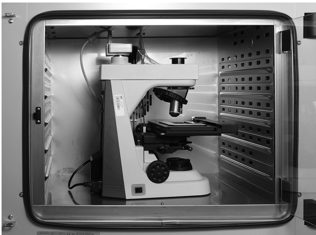
Figure 4.5: Microphotographs of the protein crystals were taken using a DS-2Mv digital camera and a remotely operated OptiScan stage attached to a Nikon Eclipse 50i microscope, which was installed in a cooled incubator ( T = 20\text{ }^{\circ}\text{C} ).
