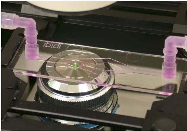
Figure 7 (origin: ibidi, Martinsried, Germany): A \mu -slide to observe the cells under flow.
