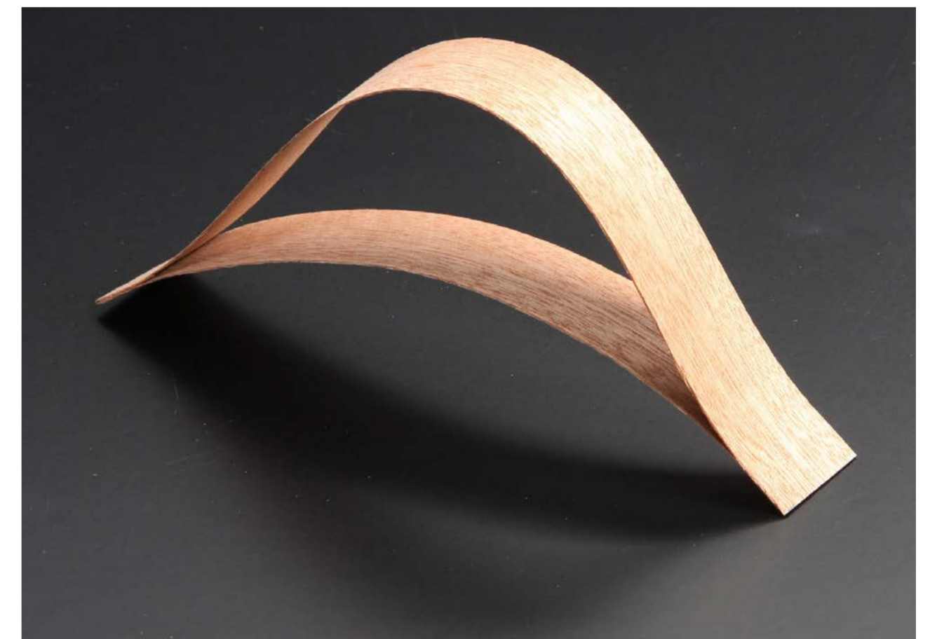
Self-stressed bow structure (J. Lienhard, ITKE Stuttgart)
