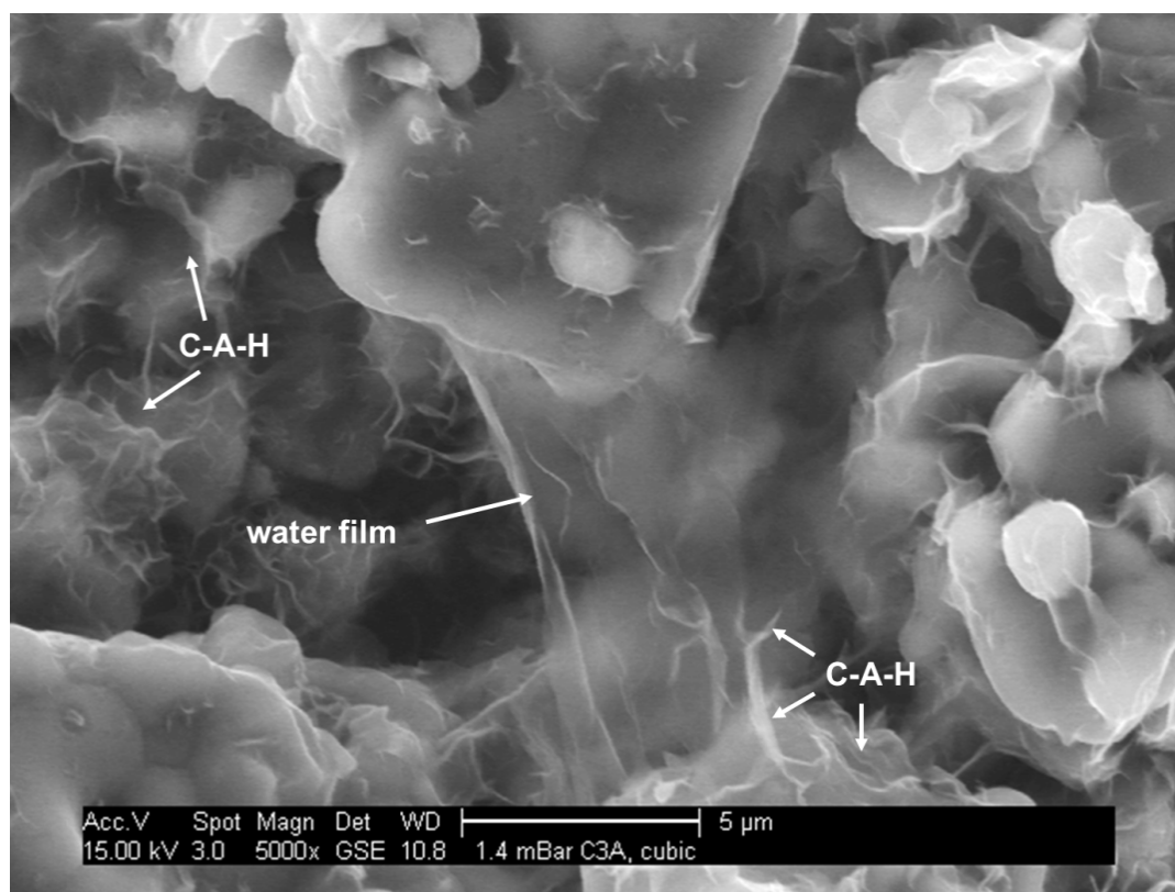
Fig. 5. ESEM image of cubic C_3A , prehydrated for 30 min in the ESEM chamber at 4.5 °C and 85 % RH, exhibiting a film of condensed liquid water between the particles.
