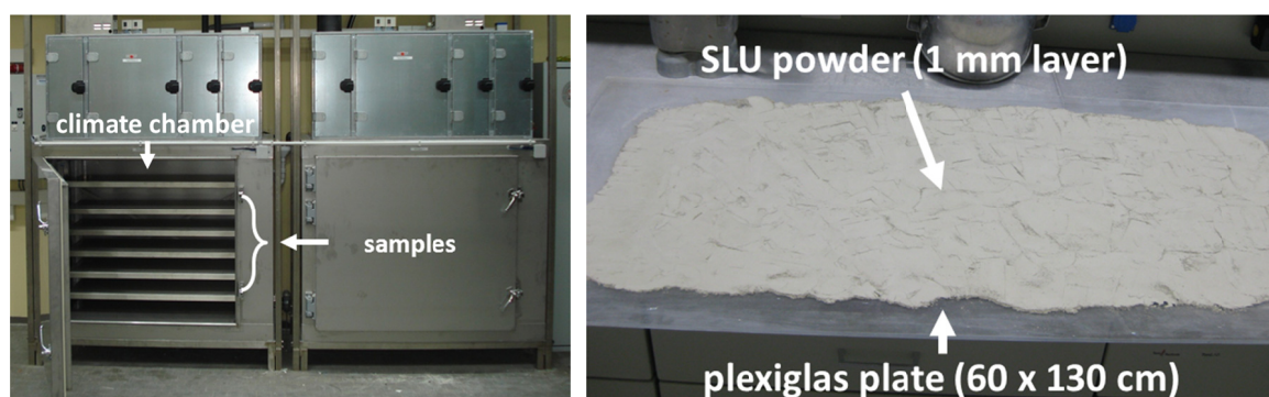
Fig. 1. Experimental set-up for ageing of the SLU in moist air: climate chamber ( left ) and thin layer of SLU powder on the plexiglas plate ( right )
