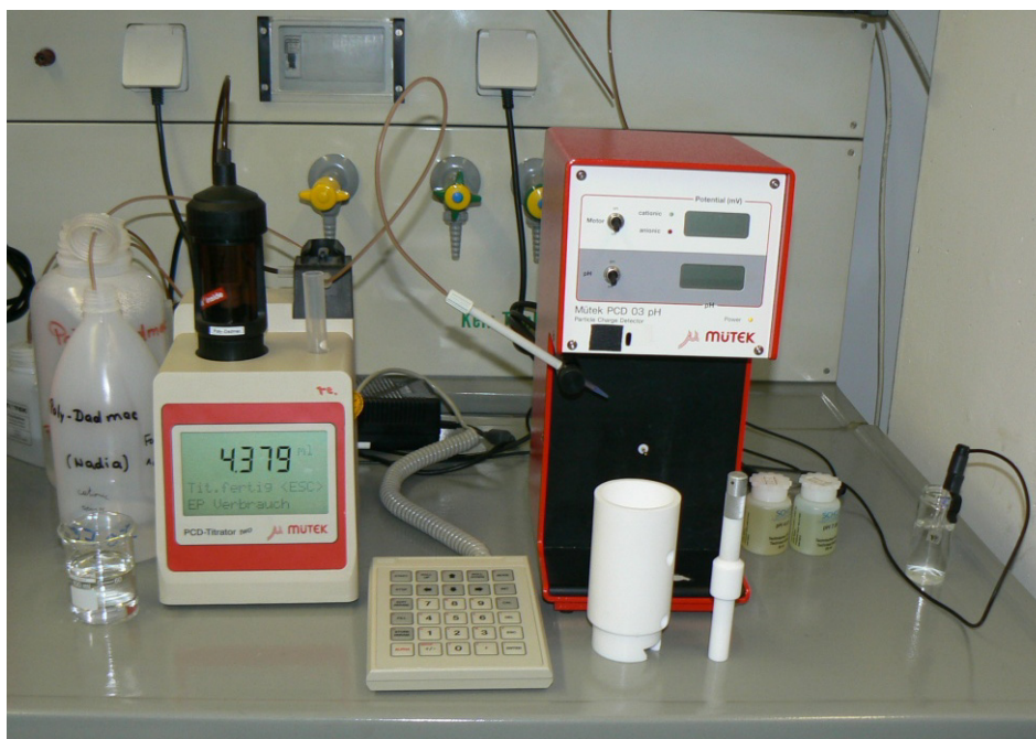
Fig. 13 Instrument used for the charge titration of polycarboxylate
