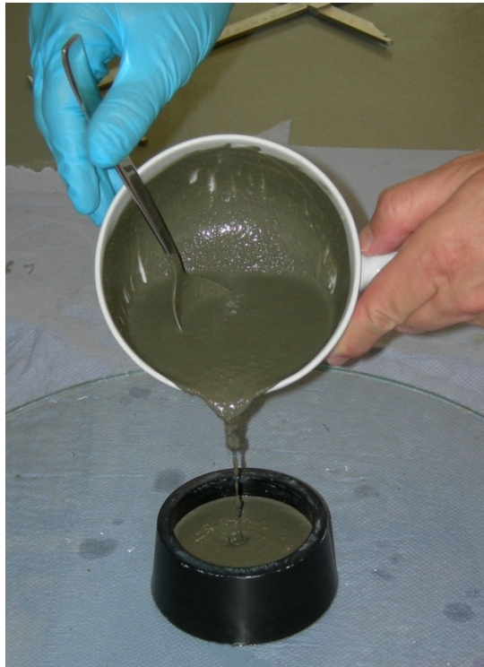
Fig. 11 Pouring a studied cement slurry into a Vicat cone on glass plate when performing the ' mini slump ' test
