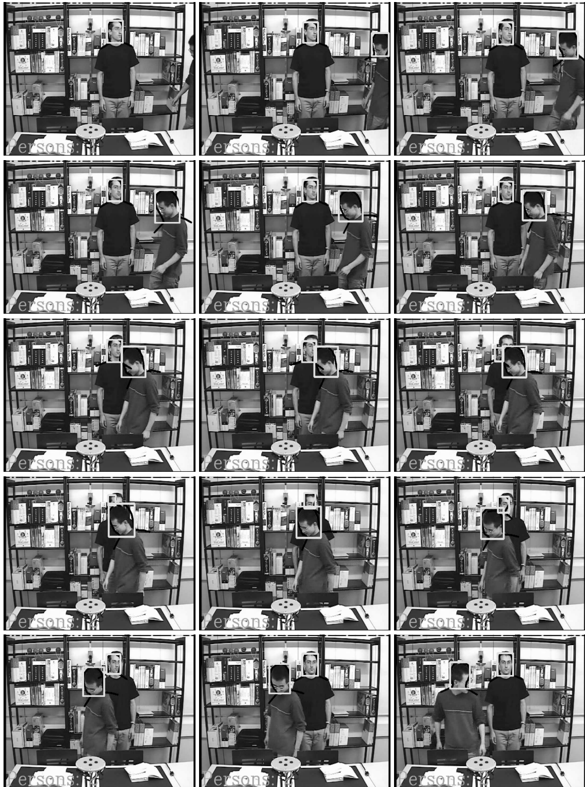
Figure 6: Meeting scenario with two persons. These exemplary frames already contain a lot of challenges like entering the room, partial occlusion and dense clutter in the background. Nevertheless the tracking output (light gray rectangles) and the number of identified tracks are very precisely.
