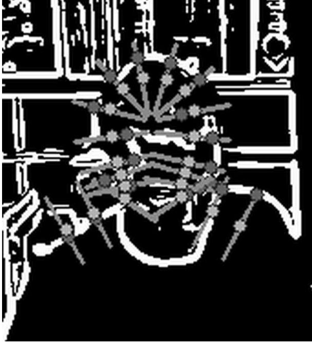
Figure 4: Gradient image, in which edges are represented by the absolute value of the gradient. Furthermore through each landmark (light gray points) the normal vectors have been plotted. Along these normals the landmarks are shifted to the pixel, where normal vector and gradient direction are most similar, resulting in the new landmark positions (dark gray points).
