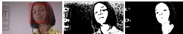
Fig. 4. Deriving skin color from the camera image. Middle: non-adaptive. Right: adaptive to the person and to the context.
