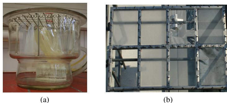
Figure A.13: Simulation of climate stress by (a) damp heat test and (b) outdoor test.
