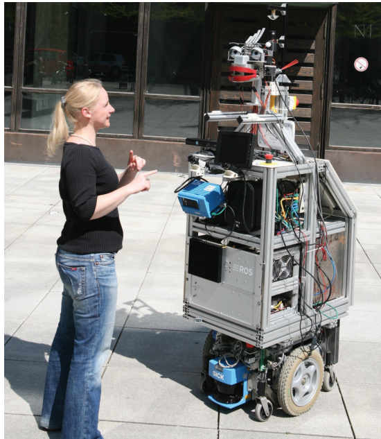
Figure 2.5: Experimental setting for the WOz-experiment: Interaction with the robot, controlled by a wizard from inside the building.
