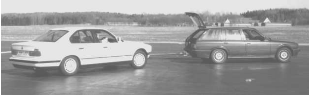
Fig. 5. Experimental setup of the vehicle convoy system
