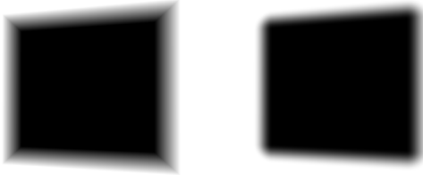
Fig.7: Pixel-based blending between views, Left: linear changeover, Right: sinusoidal changeover with rounded edges
