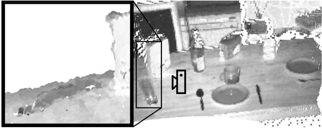
Figure 2.18: A table setting view in amplitude space (grayscale). A close-up of a glass object is shown in the left part of the figure, showing no geometry information at all. For a side view including the bottle see Figure 2.3.
