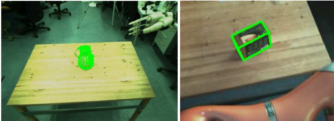
Figure 6.4: TUM-Rosie locating the resultant geometric model in an image.
