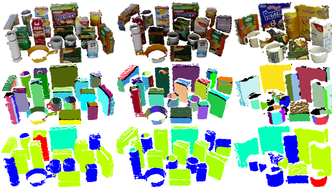
Figure 5.8: Segmentation and geometric categorization on three cluttered scenes.
