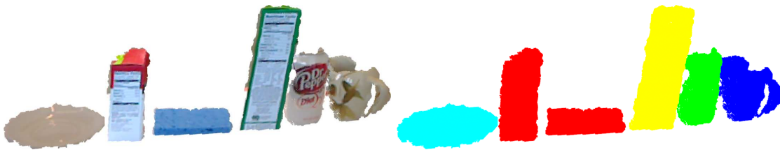
Figure 5.12: Synthetic scene automatically created and labeled from individual scans.
