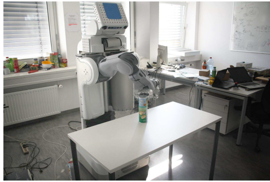
Figure 6.2: Grasping of the localized object by the PR2 robot. The fitted geometric model was triangulated and fed into the grasp planning software to obtain grasping points.
