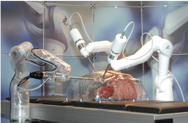
Fig. 3. Telemanipulator: three MIRO robots mounted on an operation table, white MIROs carrying MICA instruments with force/torque sensing, transparent MIRO holding a stereo endoscope.
