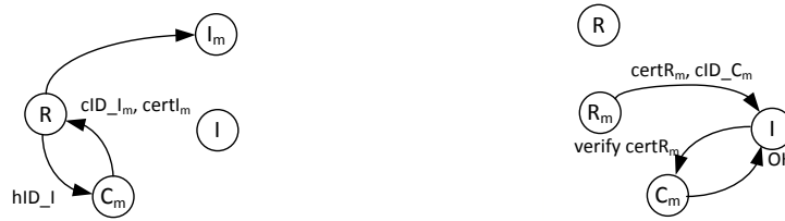
(a) Only the Counselor is malicious. R is tricked into a Trust Relationship with a faked I ( I_m ) (b) Requester and Counselor are malicious. I is tricked into a Trust Relationship with a faked R ( R_m )
