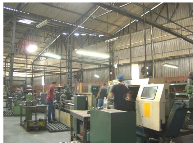
Figure 1: HDR image in Industry C - lack of integration between the equipment's layout and the lighting system.
