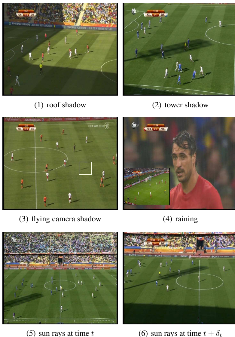
FIGURE 4.3 Examples of illumination conditions that can affect the performance of the tracker. In subfigure (1) the shadow of the roof is laying on the field, partially changing the appearance of some targets. Subfigure (2) and (3) show the shadows of other objects on the field: a tower, and a flying camera (inscribed in a white rectangle). The subfigure (4) shows a game where it was intermittently raining, causing certain change in appearance of the targets. Subfigure (5) and (6) show the effect of the Earth rotation during the course of the game, and how this changes the radiation angles from the sun rays on each target's surface. The sub-figures also show the shadows of the players due to different illumination arrangements.
