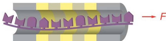
Figure 4.5: IBM nanopore sequencing approach. Single stranded DNA template strand passes through the transistor-nanopore. Individual bases are identified by unique electron signatures. Figure adapted from [88].
