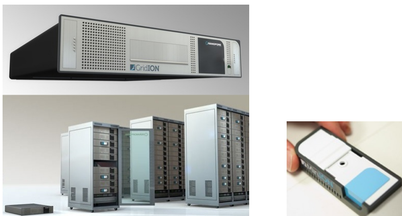
Figure 4.4: Oxford Nanopore Sequencing Instruments: GridION (single node and combined rack with multiple nodes) and MinION sequencing devices. Image available at www.nanoporetech.com .
