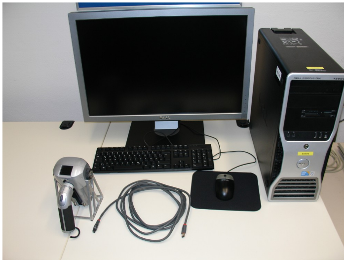
Figure C.2: Components of the multisensory DLR 3D-Modeler (ego-motion setup).
