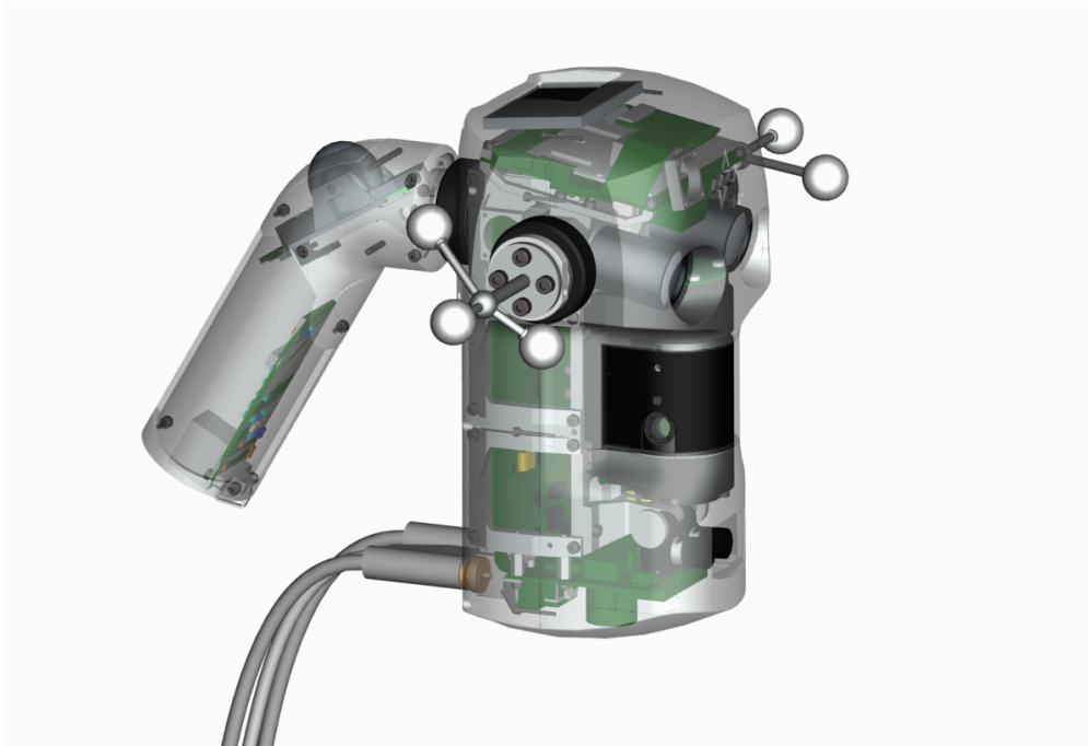
Figure 2.2: Inner view of the DLR 3D-Modeler and its electronics.
