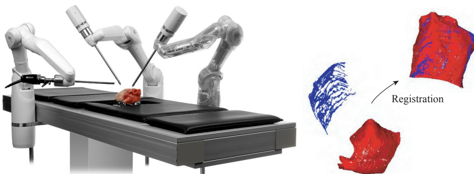
(a) The robotic system for minimally invasive surgery MiroSurge developed at DLR. (b) 3-D data registration of a torso 3-D scan using the ICP algorithm.
