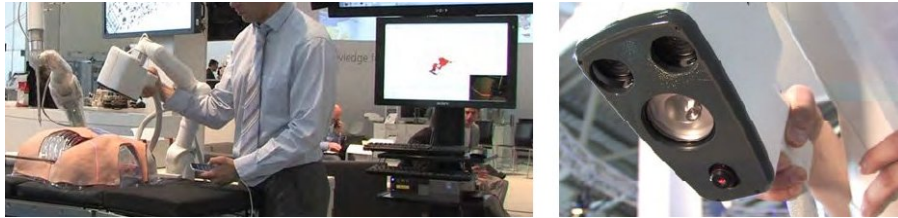
Figure B.30: The VR-Map is a hand-held perception device for robot-assisted surgery including stereo vision, an LSP, and an autopointer, refer to (Schwier et al. , 2010). It can be considered an adaptation of the DLR 3D-Modeler to medical applications (Fig. B.25 reprint).
