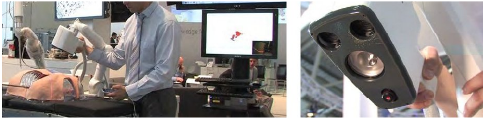
Figure B.25: The VR-Map is a device focusing on augmented reality for robot-assisted surgery including stereo vision, an LSP, and an autopointer, refer to (Schwier et al. , 2010).
