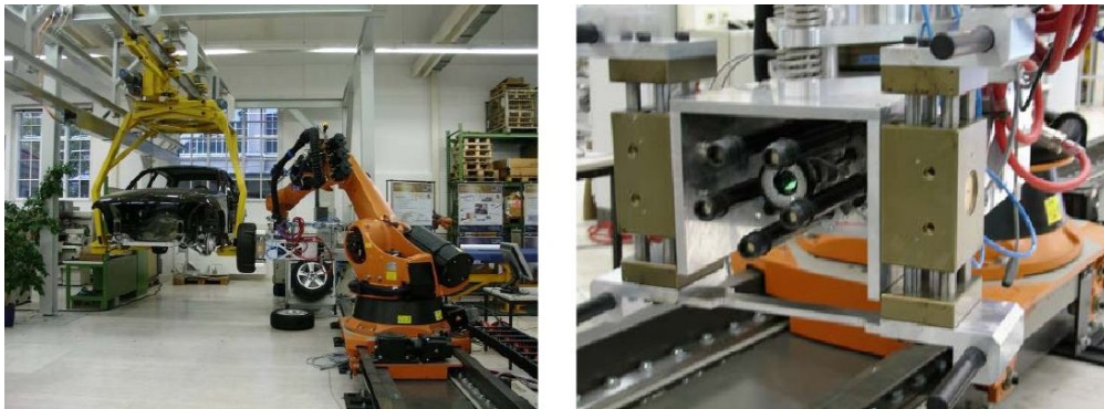
Figure B.29: Demonstration of robotic assembly of wheels onto a BMW car. In the right-hand side: close-up of the impact screwdriver mounted on the end-effector of the robot. Note the camera inbetween the five screwdriver heads.
