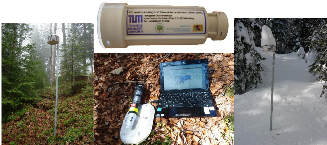
Figure 4.11 HOBO® Pro V2 Loggers (top) installed at 2 m height in solar radiation shields in the forest (left, right), reading data (bottom).
