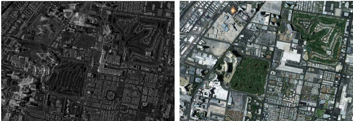
Figure 52: Mean SAR amplitude image and its corresponding Google Earth optical image of the test site Las Vegas, US.
