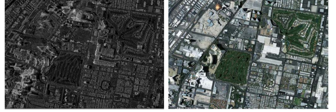
Fig. 1. Mean SAR amplitude image and its corresponding Google Earth optical image of the test site Las Vegas.
