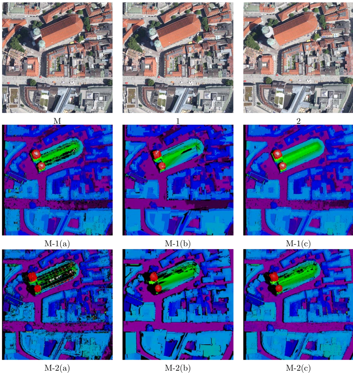
Figure 5.28: Comparison on stereo pairs with increasing baselines. M denotes the master image, which is rectified and matched with a short baseline (1) and long baseline (2) image. M-x(a) presents the results without our soft surface prior. M-x(b) are the plane-fit disparity maps to M-x(a). M-x(c) are the results with our soft surface prior.
