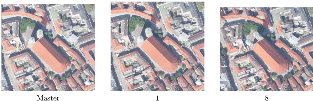
Figure 5.12: Cutdown in the church area. M denotes the master image, which is respectively matched with 1 and 8 that the stereo pair M-1 has the shortest baseline and M-8 has the longest baseline.
