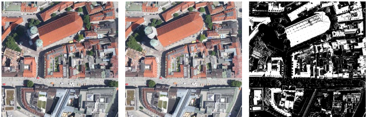
(b) Airborne stereo pair with large baseline and mask on building roofs
