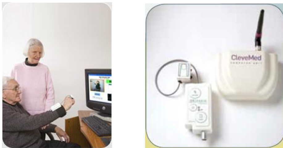
Figure 3-10: Kinesia TM (old version) for tremor and bradykinesia assessments (© CleveMed, U.S.A, 2010). On the left side of the figure, a subject performed the assessment task according to the video instruction. The right side of the figure shows the hardware of a Kinesia TM system.
