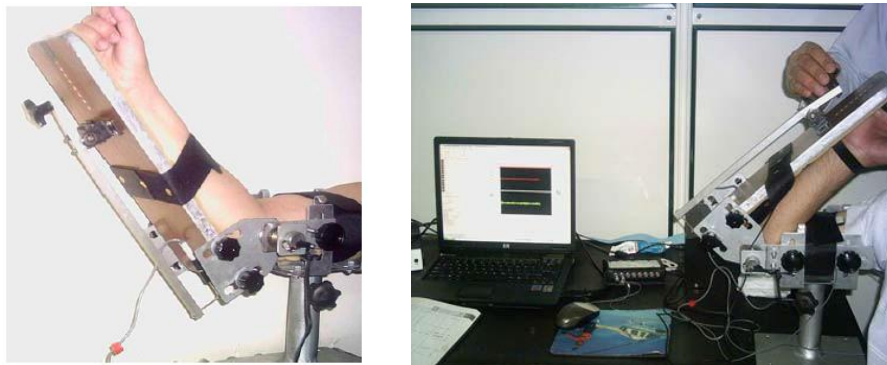
Figure 3-17: Mechanical rig test system and its operation (Taken from Sepehri et al. , 2007). The elbow movement was driven by an examiner.
