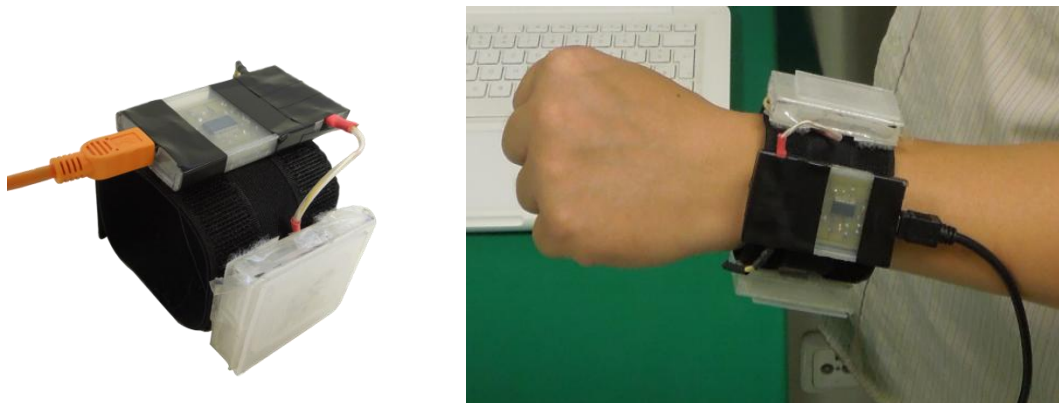
Figure 6-31: Overview of the prototype for rigidity assessment (Based on Dai et al. , 2013b).
