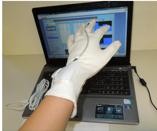
Figure 6-26: Tremor/bradykinesia assessment system.
