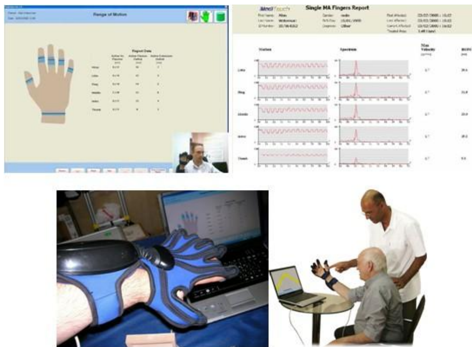
Figure 3-12: HandTutor TM . Electro-optical sensors, bend sensors, and accelerometers are placed in the upper side of each finger. The training parameters of each finger are displayed in the GUI. It is power supplied by the USB interface of a computer (© MediTouch, 2010).
