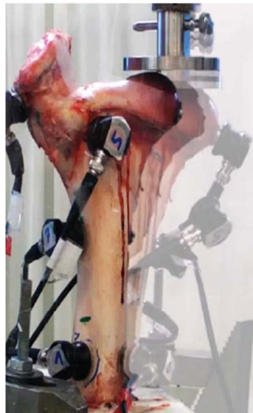
Figure 1: Compressional testing of a bovine bone; from [1]
