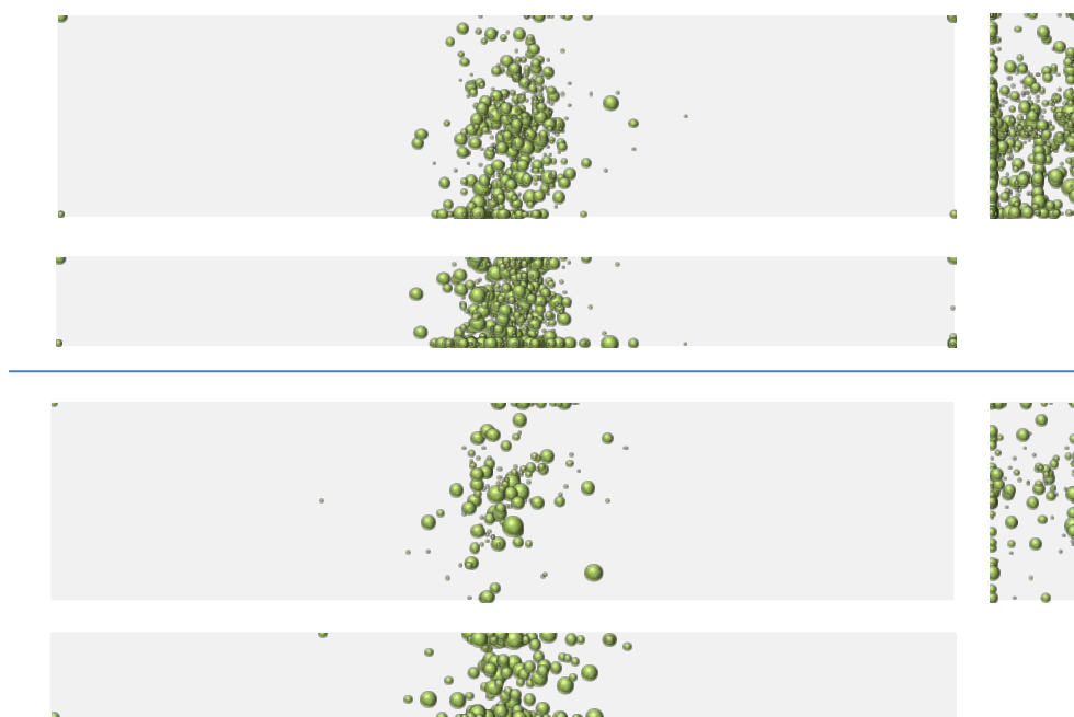
Figure 2: Acoustic emission activity recorded before (top) and after (bottom) healing of the specimen shown in fig. 1 (Van Tittelboom et al. 2012)
