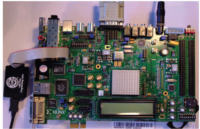
Fig. 4. Test set-up with FPGA development board, with JTAG connection (left) to the application processor debug support unit and serial connection (top) to that of the HSM processor.
