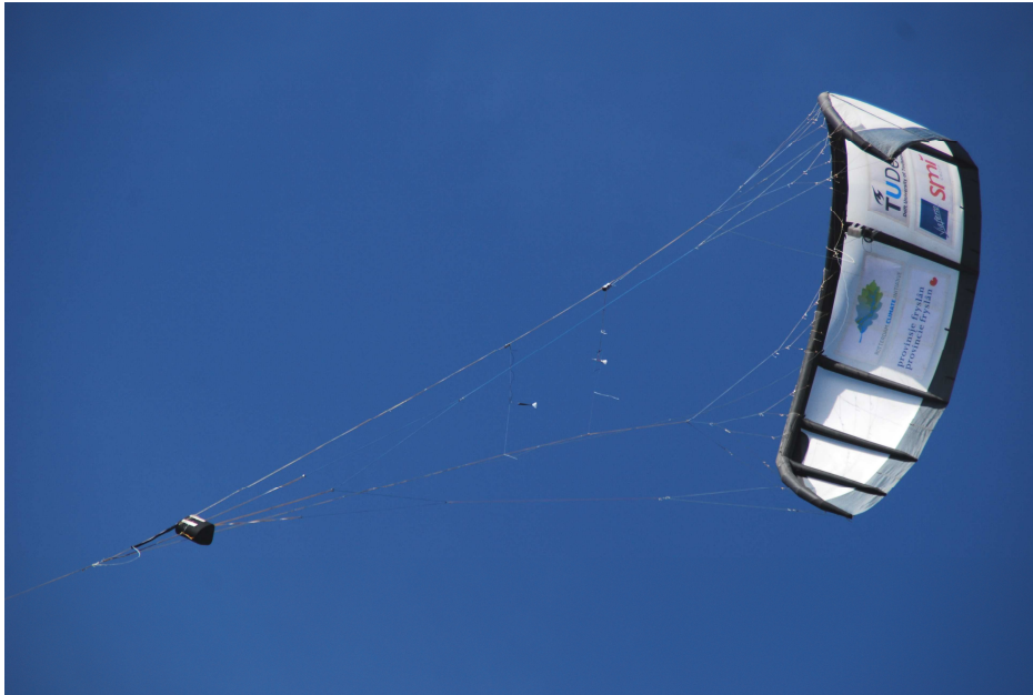
Figure 2-3: An airborne LEI-type [16]; in the lower left corner the control pod can be seen, while the PITO-tube is suspended between the bridle lines
