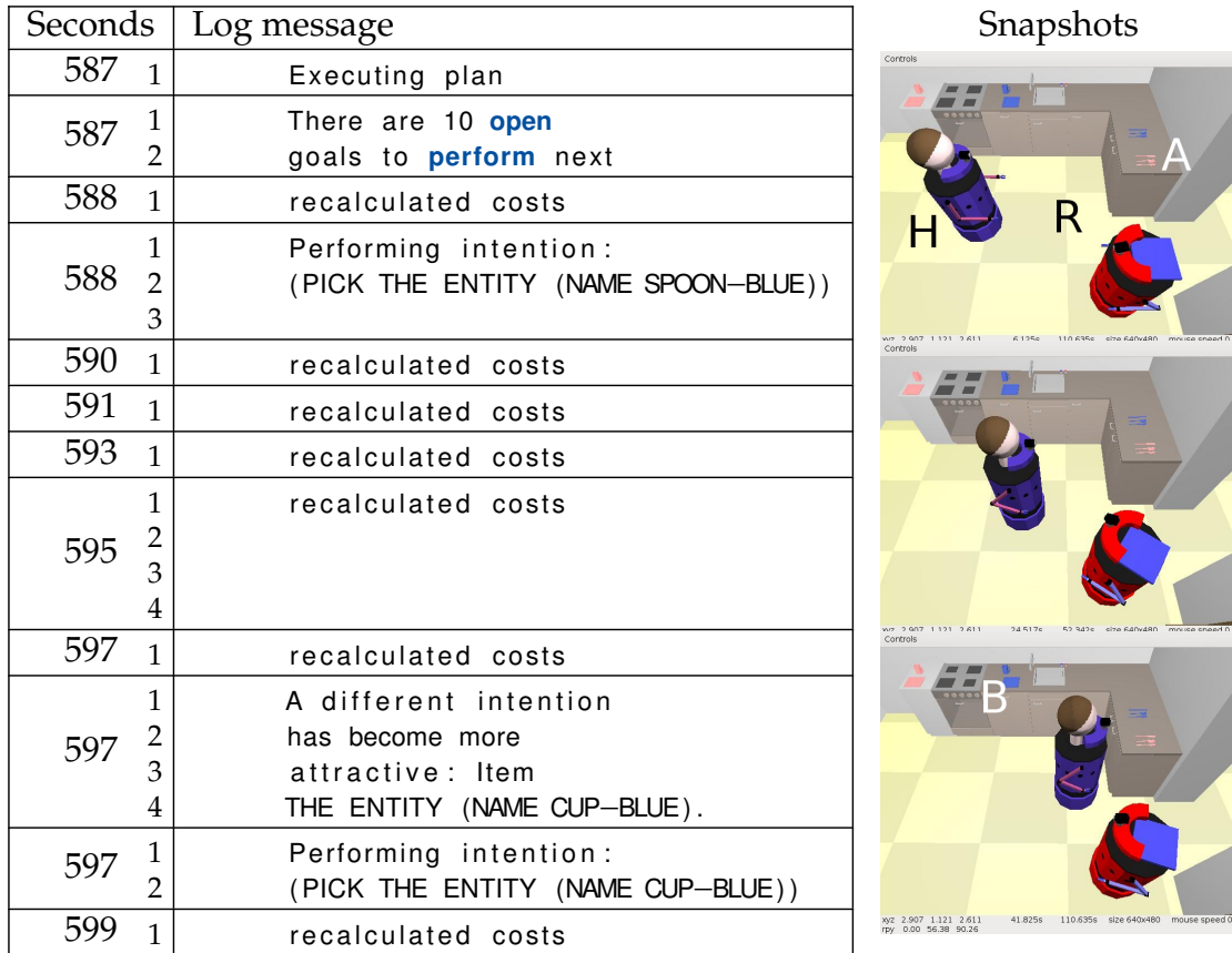
Figure 4.11: Logfile and snapshots showing opportunistic change of intention due to spatial circumstance. At time 588 the robot R decided to next pick item SPOON-BLUE shown as location A, and at time 597, the robot instead decided to pick item CUP-BLUE at location B, EVEN though SPOON-BLUE was still closer given Euclidean distance, but has higher path costs due to the human H having moved.
