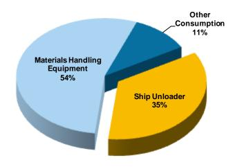
Fig. 3: Breakdown of the Power Consumption of an Import Terminal
