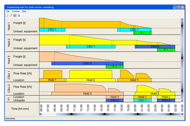
Fig. 5: Mock-up of the auxiliary tool for planning the unloading procedure (CSU: Continuous ship unloader; F: Feeding device)
