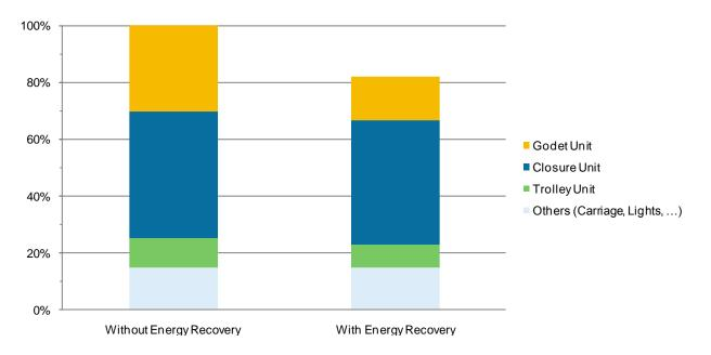
Fig. 4: Breakdown of the Power Consumption of a Gantry Crane with and without Energy Recovery
