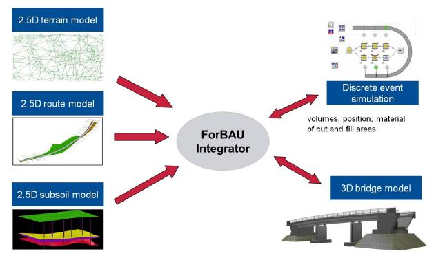
Fig. 2: The ForBAU integrator linking various submodels of the digital construction site together (Günthner and Borrmann, 2011)
