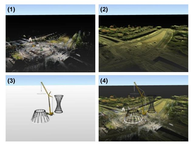
Fig. 10: (1) point cloud of terrestrial laser scanning, (2) point cloud of airborne measurements, (3) parametric 3D model of the crane and the sculpture, (4) point clouds merged with 3D models (ForBAU, 2011)
