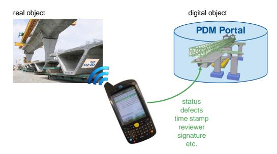
Fig. 7: Concept of mobile building data transmission
