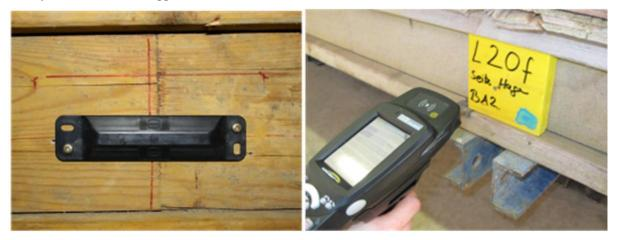
Fig. 6: Labeled modular shuttering systems (hard tag on the left, Smart Label on the right)
