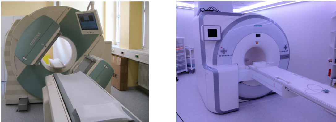
Figure 1.11: Big tomographic systems like SPECT/CT (left) and PET/MR (right) are used in diagnostics to acquire 3D images of the patient with high accuracy.
