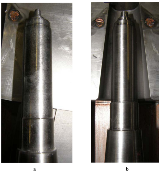
FIG. 26. (Color online) Tools for injection molding of Al-alloys for automotive industry after the fabrication of 15 000 parts. The length is about 200 mm and diameter 15–25 mm. (a) Conventionally treated by plasma nitriding, which forms several 10 μm thick layer, (b) coated with 2–3 μm thick layer of nc-(Cr 1-x Al x )N/a-Si 3 N 4 nanocomposite (Ref. 292).
