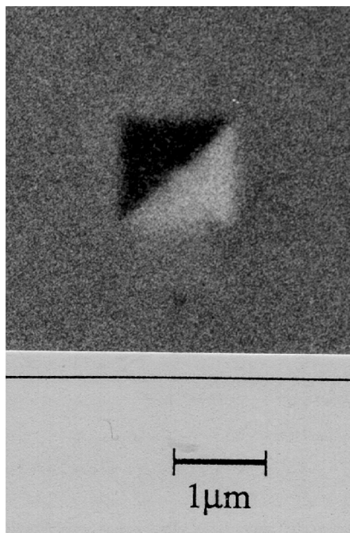
Fig. 14. Scanning electron micrograph of an indentation into about 8 \mu\text{m} thick, long-term stable quasibinary nc-TiN/a-Si 3 N 4 nanocomposite coating with a Vickers diamond indenter at a load of 110 mN. The magnification of the scanning electron microscope has been calibrated using a photomask for optical lithography in semiconductor industry. One notices that the plastically deformed indentation area of 1 \mu\text{m}^2 ( = 10^{-12} m 2 ) produced under a load of 100 mN corresponds to a Meyer's hardness of 0.1 N/10 -12 m 2 = 10 11 N/m 2 = 100 GPa. Reprinted with permission from Vepek and Vepek-Heijman, Thin Solid Films 522 , 274 (2012). Copyright 2012, Elsevier B.V.
