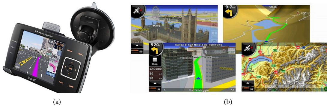
Figure 2.14: (a) Samsung STT-D370 (2007) for Korea was the first to display photo realistic 3D city maps. (b) Clarion Map 780 (2008) introduced 3D landmarks, buildings and a DEM.
