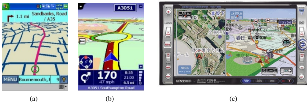
Figure 2.13: (a) Destinator 2 from PowerLOC Technologies (2002) is the first system to display a 2.5D birds-eye-view map. (b) TomTom Navigator 2 (2002) enhances the 2.5D view with land-cover and POIs. (c) Kenwood HDD navigation HDV-910 (2004) introduces satellite imagery.
