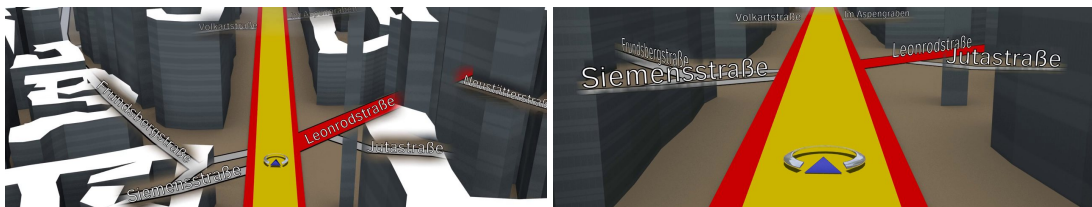
Figure 5.5: Transparency label aura: labels create a transparent region in the occluding objects in bird's eye with SS (left) and snail's view with WS labeling (right).
