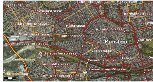
(b) Labeling of a road network in a GIS. In this figure, we define a large buffer zone around the labels to enhance readability and visual association.
