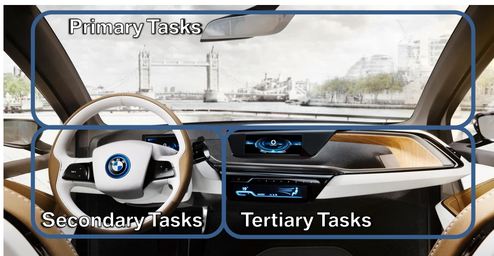
Figure 2.16: Fully integrated displays in modern cars assist the driver to perform interactive tasks [TBK06]. (top) The Head-Up-Display in the windshield helps performing the primary task, i.e., driving. (bottom left) The instrument cluster assists secondary tasks, e.g., activating turning signals or displaying guidance information. (bottom right) The dashboard assists tertiary tasks, i.e., entertainment, orientation or information, e.g., searching POIs.
