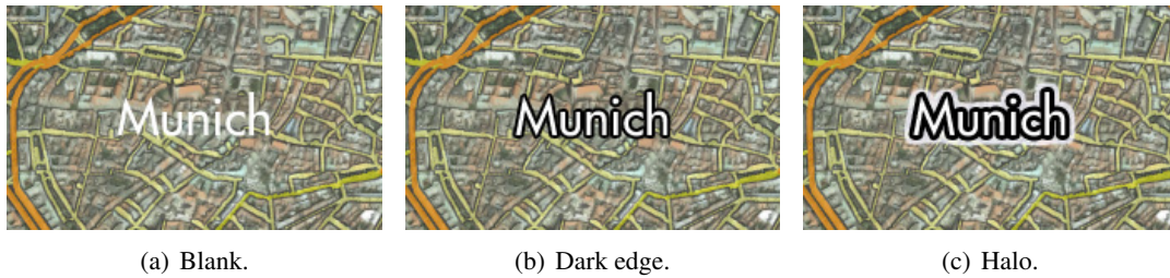
Figure 4.7: Techniques for increasing the readability of annotations. The best readability is achieved by adding an outline and a halo around the label.
