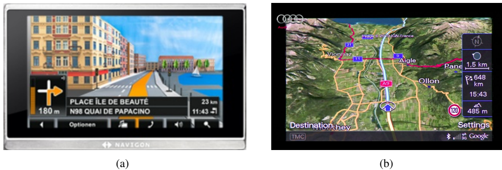
Figure 2.15: (a) Navigon 8410 features complete 3D city models for the European and US market. (b) Audi A8 streams high-resolution satellite imagery from Google's back-end server (courtesy of AUDI AG).
