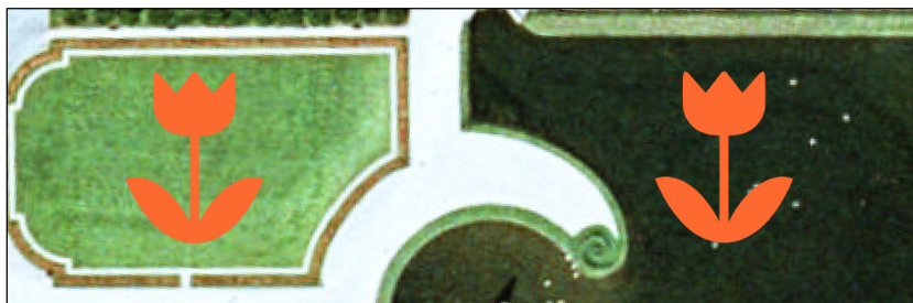
Figure 4-11 - The simultaneous contrast effect on imagery: Both flower symbols have the same colour hue, tone, and saturation. Nonetheless, their visual appearance is different.
