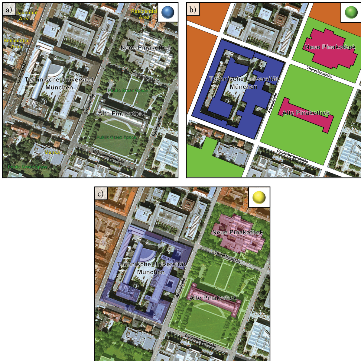
Figure 3-18 - Different design examples of image maps between realism and abstraction: a) high degree of labelling – zero symbolisation, b) medium degree of labelling – high symbolisation degree – zero symbolisation transparency, and c) medium degree of labelling – high symbolisation degree – high symbolisation transparency
