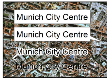
Figure 1-16 - Contrast improving type effects; from top to down: rectangle box, callout, halo, drop shadow
