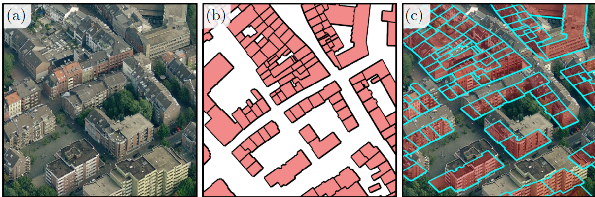
Figure 1-13 - A set of oblique aerial images (a), a cadastral map (b), and the registration of images (c), (Habbecke and Kobbelt, 2012).
