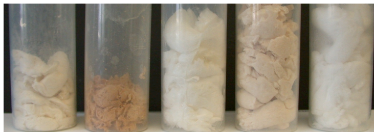
Figure 3.2 – Isolated EPS from different strains. From left to right: G. cerinus , G. oxidans , G. frateurii , N. chiangmaiensis , K. baliensis . Starter culture was grown overnight in GM-medium and main culture in 200 ml NaG-medium with 100 g/l sucrose, incubated at 30 °C and 180 rpm for 48 h.
