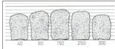
Figure 1.1 – Relation between energy input during kneading and loaf volume of baked wheat bread. x-axis: kneading energy (kJ/kg). After Frazier et al. ([Frazier et al., 1979])
