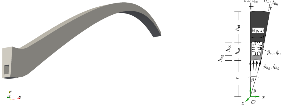
Figure 7.25: Rocket nozzle: initial geometry and prescribed boundary conditions. Three-dimensional view of the considered geometry containing one cooling channel (left) and cross section with the definition of dimensions and loads (right).
