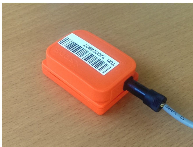
Figure 4.3: XSens gyroscope retrieves accurate orientation data with low latency.
