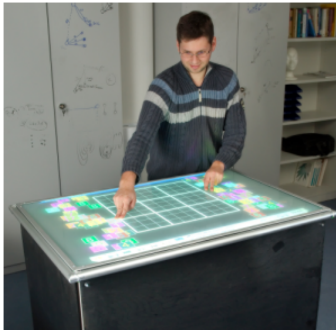
Figure 4.5: Tangible Interaction Surfaces for Collaboration between Humans (TISCH) multi-touch device.
