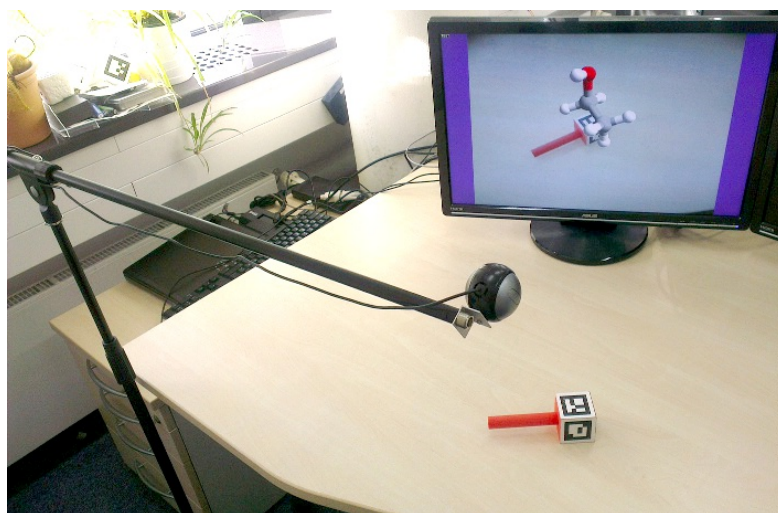
Figure 4.7: To give the user as much space to move, I used a microphone stand with the camera mounted at the end of the arm.
