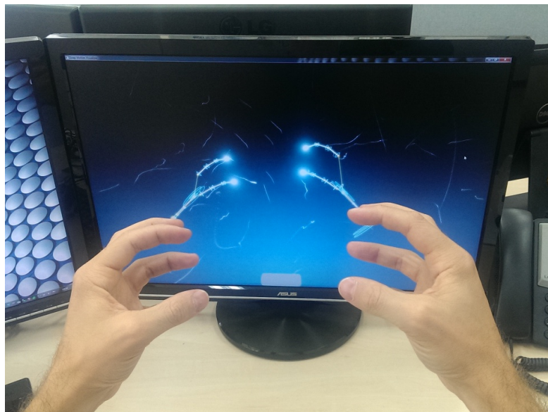
Figure 4.4: Finger tracking of the LEAP Motion gives orientation and position data of the two hands.
